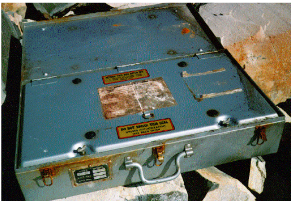
Figure 8 Inner lid on aluminum "Explosives" box
